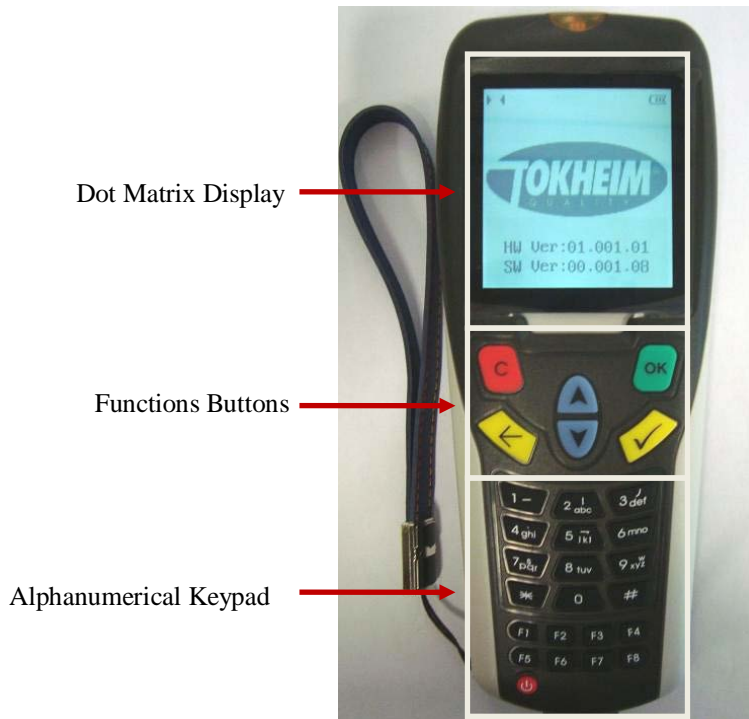
Figure 7 Main functions of Hand Held Terminal (HHT)
