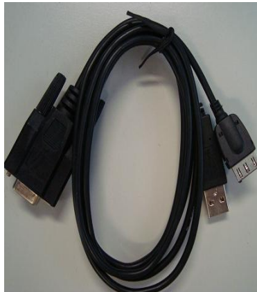
Figure 5 Serial port RS-232 with USB connection
